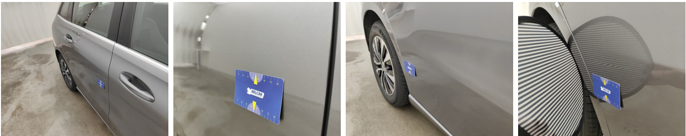
Door Rear Right // Repair & Painting-scratch + dent
