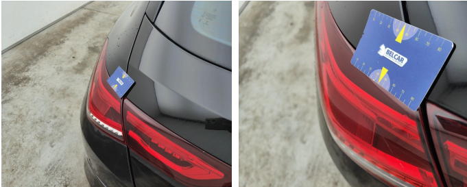
Light / Rear left / Replace-scratch
