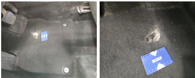
Interior / Floor Covering / Replace-hole
