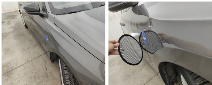
Wing Front right // Painting-bad repair
