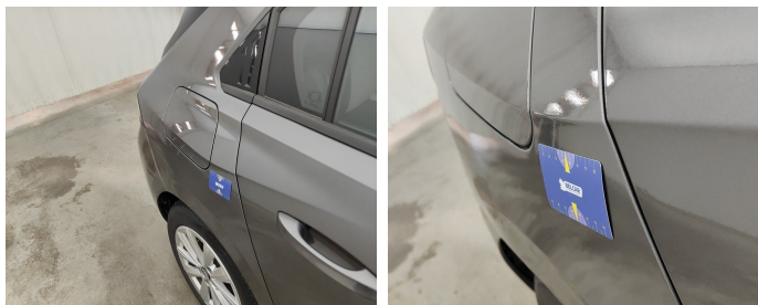
Wing Rear Right // Painting-bad repair
