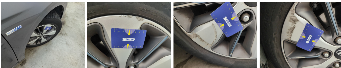
Wheel Alloy Front Right // Repair-scratch
