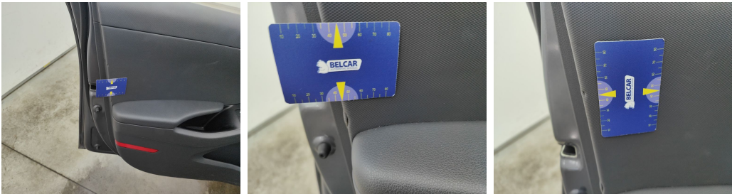
Front Left Door Interior Coating // Replace Completely-tear
