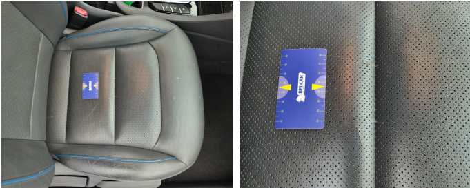
Seat Front Right / Bottom Coating / Replace-worn
