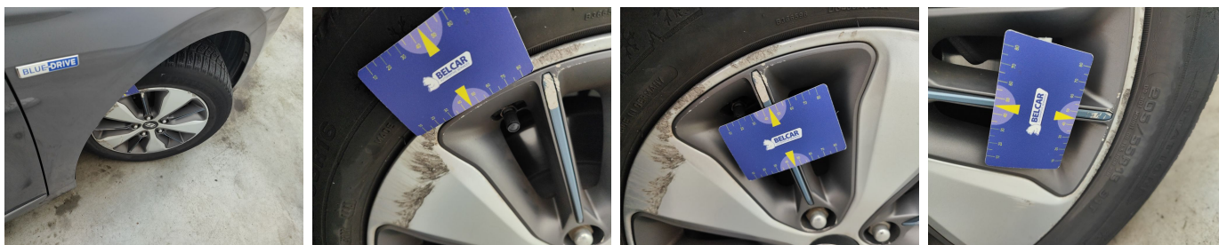
Wheel Front Right / Wheel Cover / Replace-scratch
