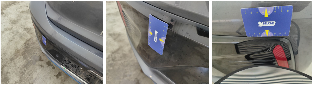
Bumper Rear / Trim Center / Replace-scratch + dent
