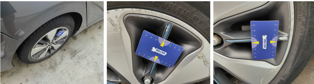
Wheel Rear Right / Wheel Cover / Replace-scratch
