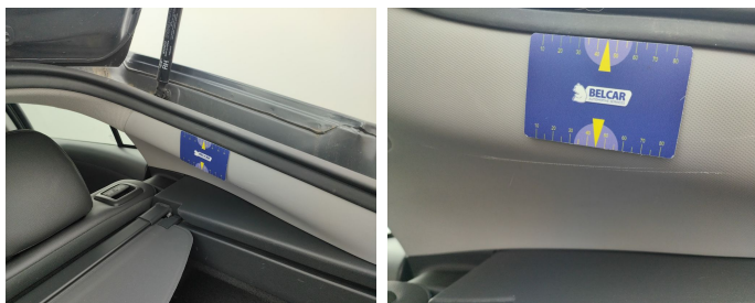
Trunk Compartment / Side Cover Right / Replace-scratch
