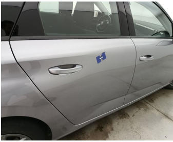
Door Rear Right // Repair & Painting-scratch + dent
