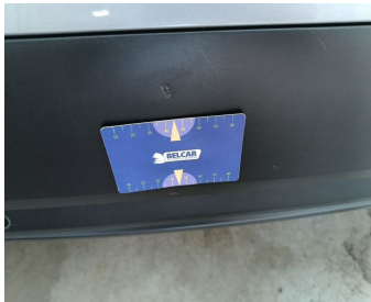
Bumper Rear / Lower Cover Not Painted / Replace-scratch
