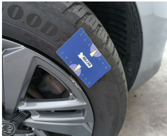
Wheel Alloy Front Right // Repair-scratch
