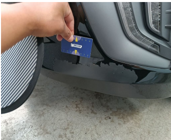
Bumper Front // Painting-bad repair
