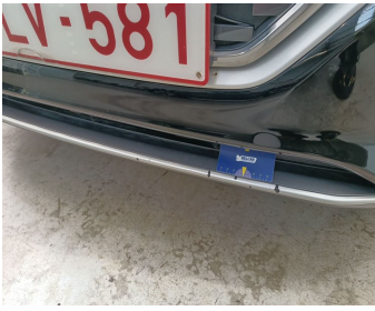
Bumper Front / Spoiler / Replace-bad repair
