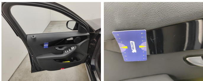
Front Left Door Interior Coating // Replace Completely-scratch
