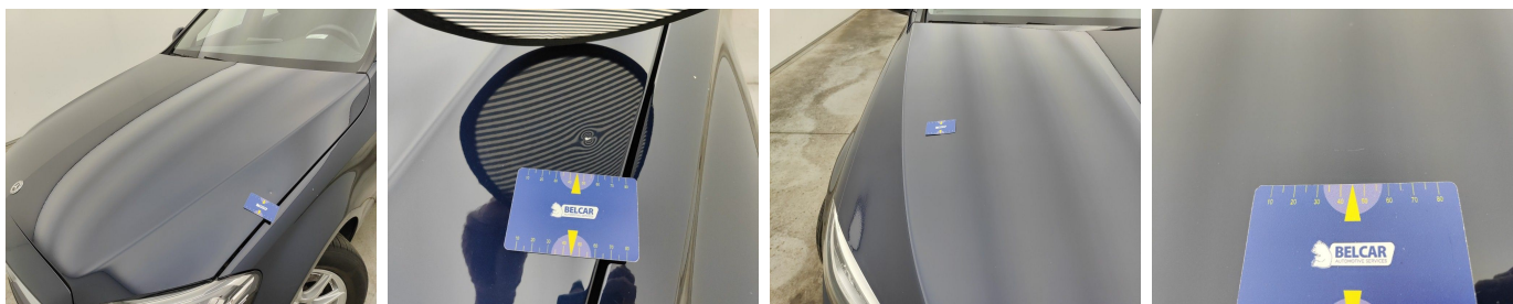
Front Bonnet // Repair & Painting-scratch + dent
