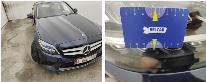
Light / Front Right / Replace-scratch
