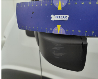
Side View Mirror Left / Shell / Replace Not Painted-scratch
