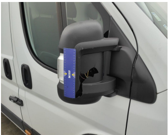
Side View Mirror Right / Shell / Replace Not Painted-cracked
