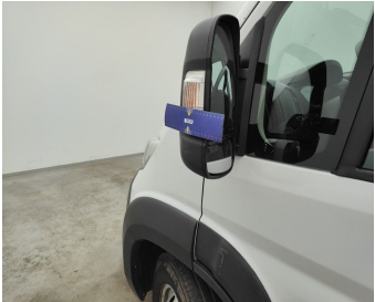
Side View Mirror Left / Shell / Replace Not Painted-scratch
