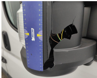
Side View Mirror Right / Shell / Replace Not Painted-cracked
