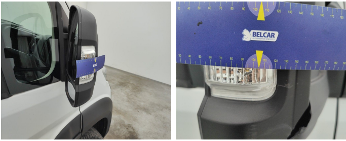
Side View Mirror Right / Direction Indicator / Replace-cracked
