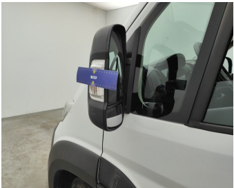
Side View Mirror Left / Direction Indicator / Replace-scratch
