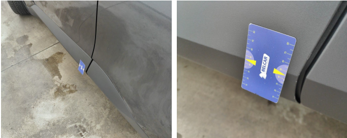
Door Front Left / Trim / Replace-scratch
