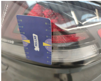
Light / Rear Right On Rear Bonnet / Replace-cracked
