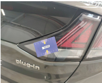
Light / Rear Right On Rear Bonnet / Replace-cracked
