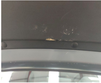
Front Bonnet / Insulation / Replace-tear
