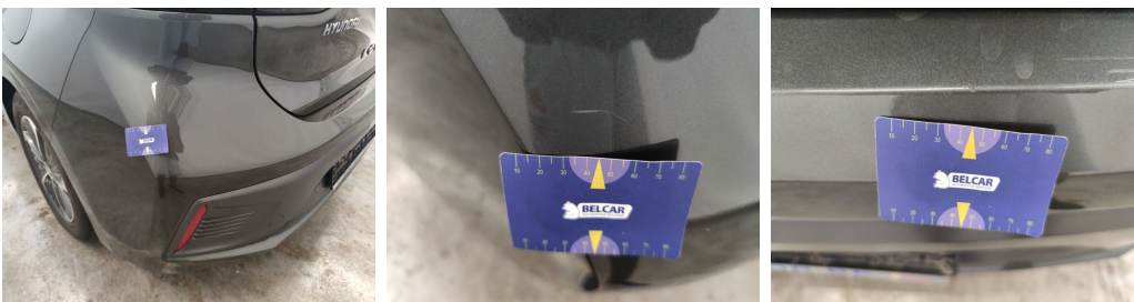
Wing Rear Left // Smart Repair Small-dent
