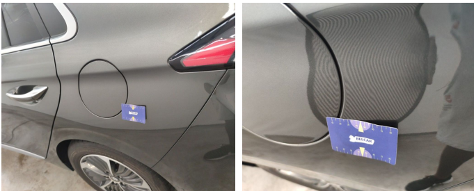
Wing Rear Left // Smart Repair Small-dent
