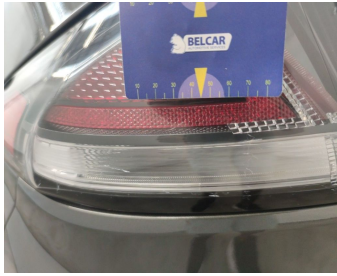
Light / Rear Left On Rear Bonnet / Replace-cracked
