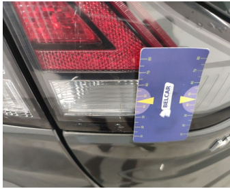
Light / Rear Left On Rear Bonnet / Replace-cracked
