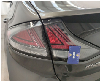
Light / Rear Left On Rear Bonnet / Replace-cracked
