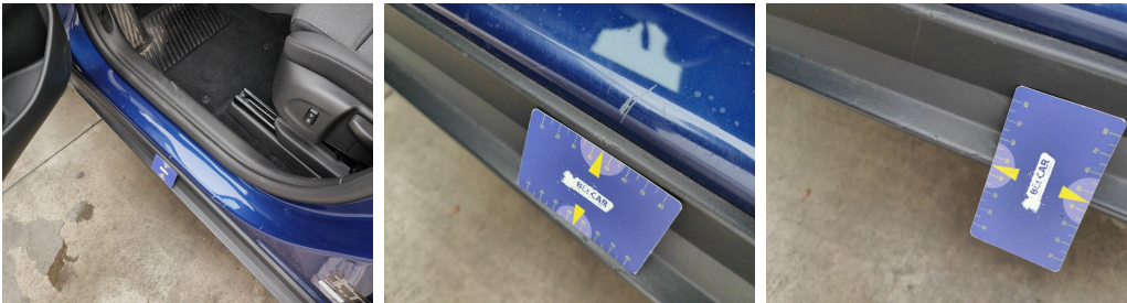
Rocker Panel Left / Cover Not Painted / Replace-scratch
