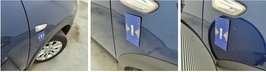
Wing Front right // Painting-bad repair
