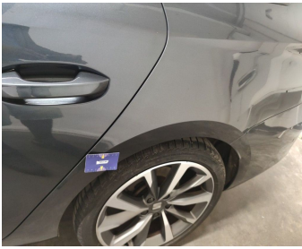
Wing Rear Left // Smart Repair Medium-scratch
