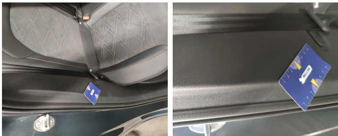
Interior / Side Cover rear Seat / Replace-scratch
