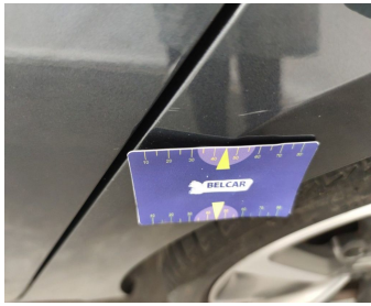
Wing Rear Left // Smart Repair Medium-scratch
