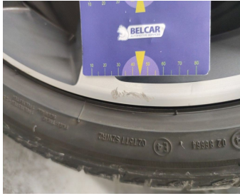
Wheel Two Tone Front Left // Repair-scratch
