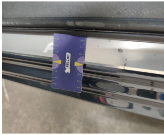
Rocker Panel Left // Smart Repair Medium-dent
