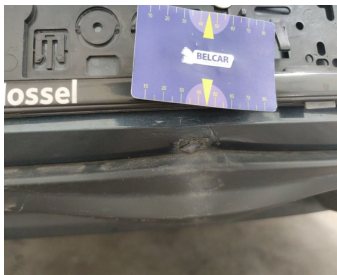
Bumper Rear // Repair & Painting-cracked
