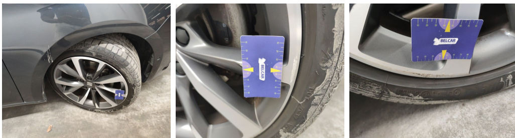
Wheel Two Tone Front Right // Repair-scratch
