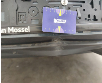
Bumper Rear / Lower Cover Not Painted / Replace-scratch + dent
