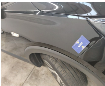
Wing Front right // Repair & Painting-bad repair
