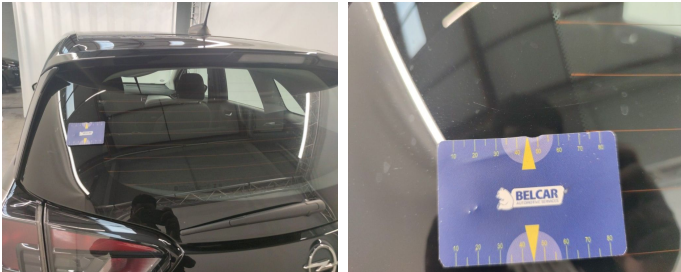
Rear Bonnet / Rear Window / Replace-scratch
