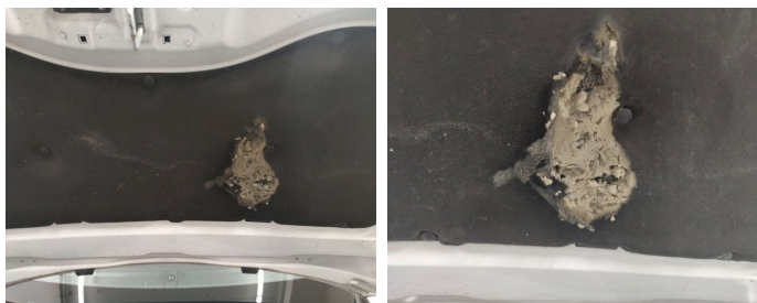
Front Bonnet / Insulation / Replace-cracked
