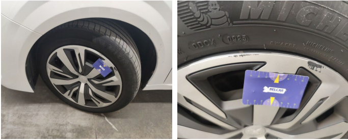
Wheel Front Left / Wheel Cover / Replace-scratch
