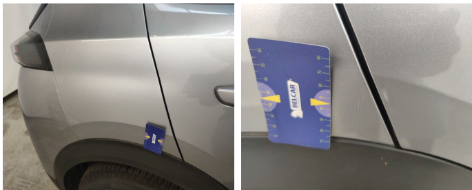
Wing Rear Right // Smart Repair Medium-scratch
