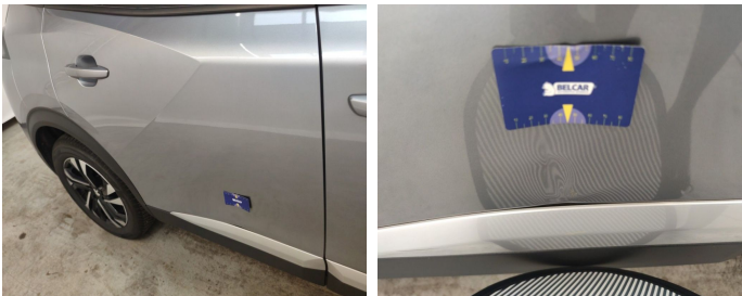
Door Rear Right // Repair & Painting-scratch + dent
