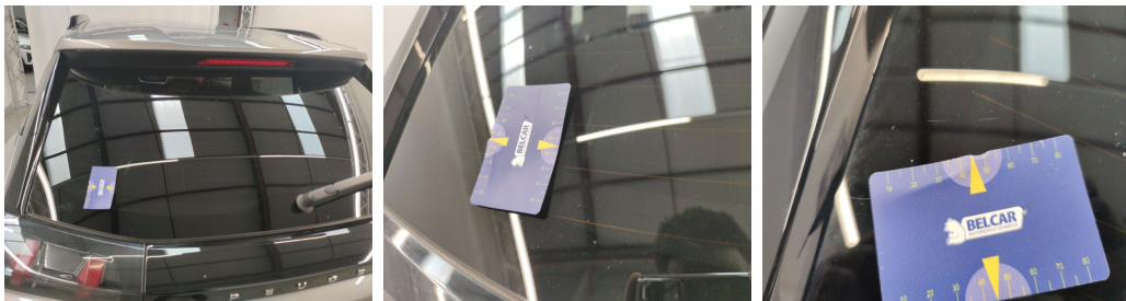
Rear Bonnet / Rear Window / Replace-scratch
