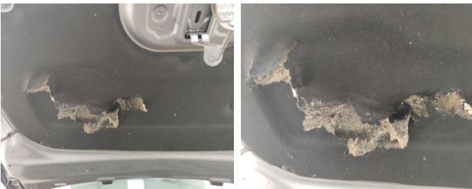
Front Bonnet / Insulation / Replace-cracked
