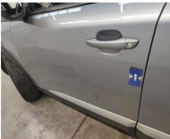
Door Front Left // Smart Repair Medium-scratch
