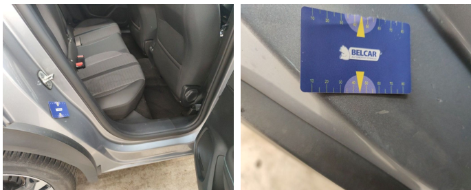
Rocker Panel Right // Smart Repair Medium-scratch
