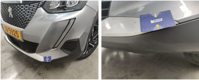
Bumper Front / Lower Cover Not Painted / Replace-scratch
