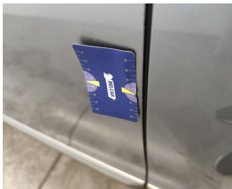
Door Front Left // Smart Repair Medium-scratch
