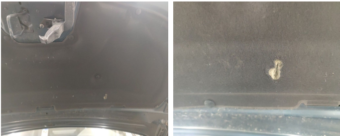
Front Bonnet / Insulation / Replace-cracked
