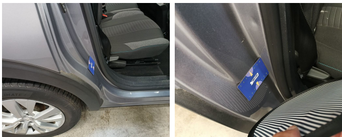
Rocker Panel Right // Smart Repair Medium-scratch + dent
