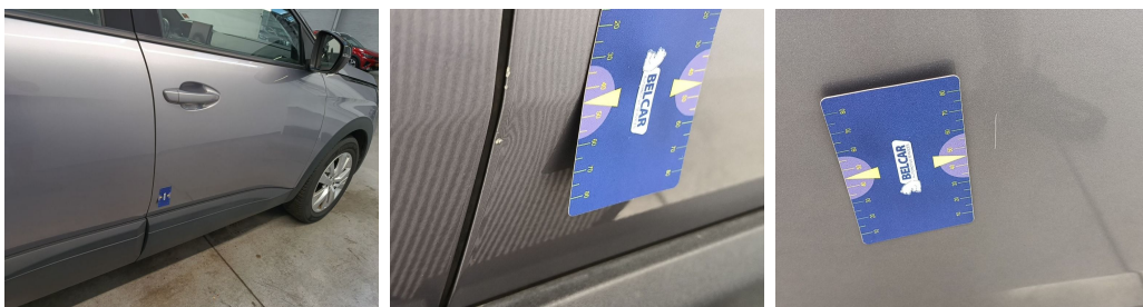
Door Front Right // Smart Repair Medium-scratch + dent
