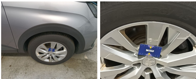
Wheel Alloy Front Right // Repair-scratch
