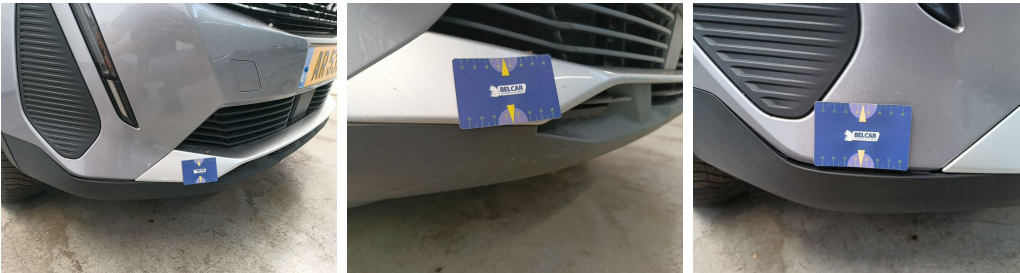
Bumper Front / Lower Cover Not Painted / Replace-scratch + dent
