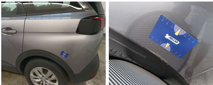
Wing Rear Left // Repair & Painting-scratch + dent
