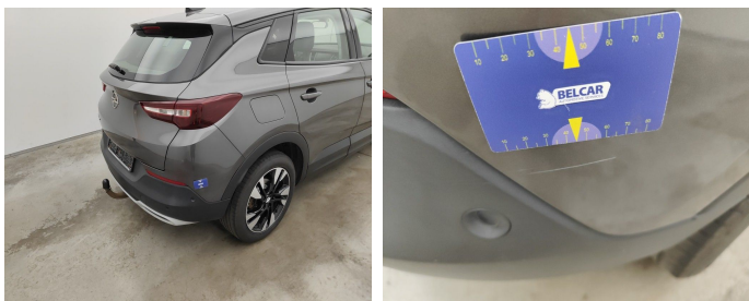
Bumper Rear // Painting-scratch
