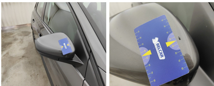
Side View Mirror Right // Painting-scratch
