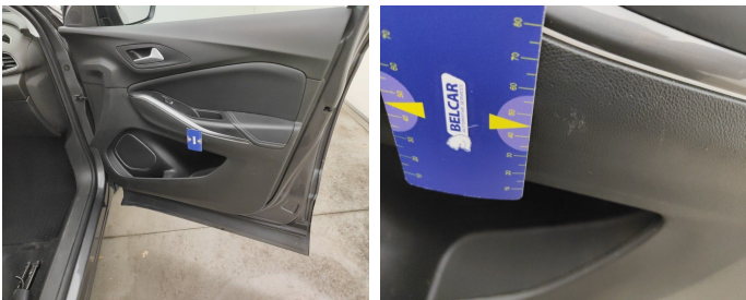
Front Right Door Interior Coating // Replace Completely-scratch
