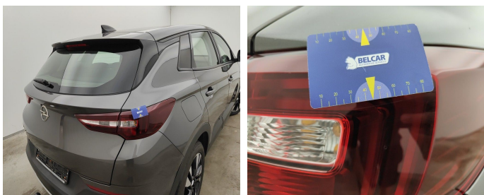
Light / Rear Right / Replace-scratch
