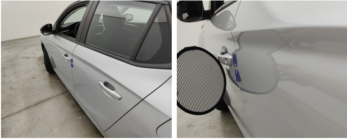
Door Rear Left // Smart Repair Small-dent
