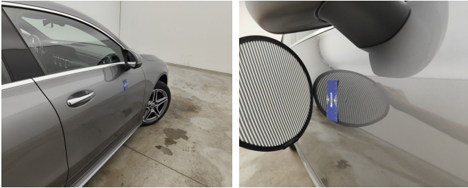
Door Front Right // Smart Repair Small-dent
