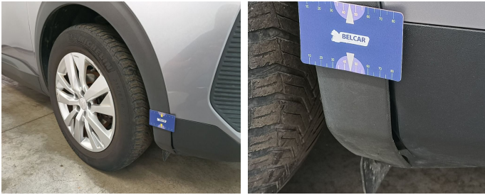
Wing Front right / Trim / Replace-scratch + dent
