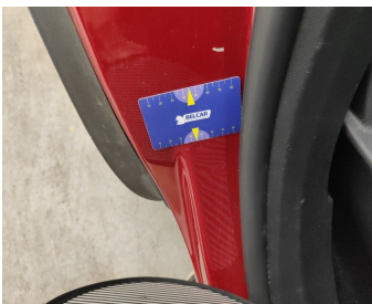
Rocker Panel Right // Smart Repair Medium-scratch + dent
