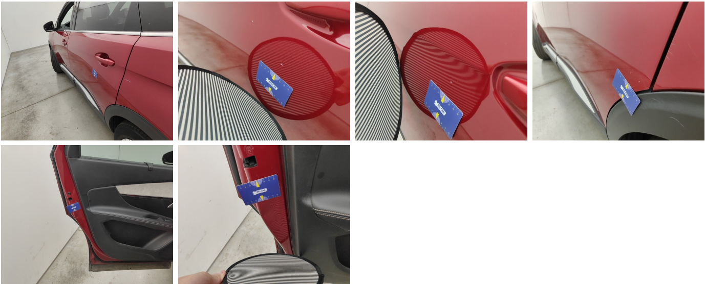
Door Rear Left // Repair & Painting-scratch + dent
