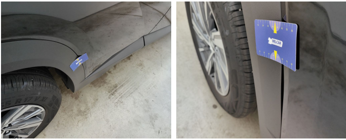
Wing Rear Right / Trim / Replace-bad position
