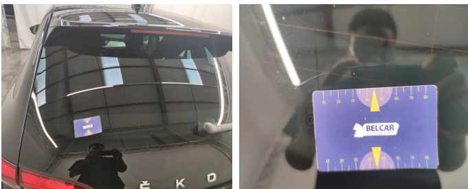
Rear Bonnet / Rear Window / Replace-scratch
