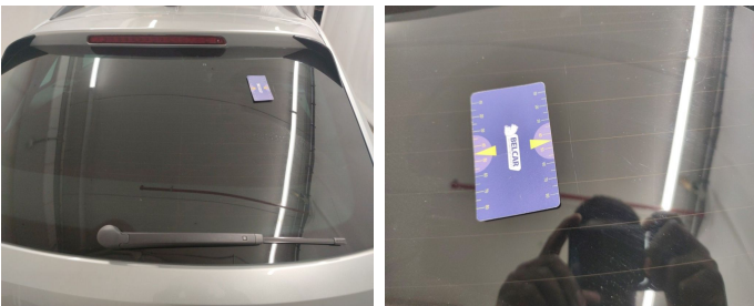
Rear Bonnet / Rear Window / Replace-scratch
