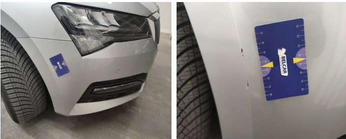
Bumper Front // Smart Repair Large-scratch
