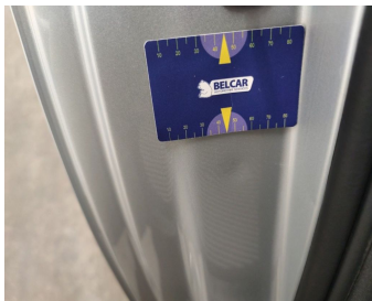
Rocker Panel Right // Smart Repair Medium-scratch + dent
