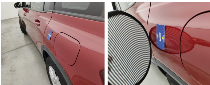
Wing Rear Left // Smart Repair Small-dent
