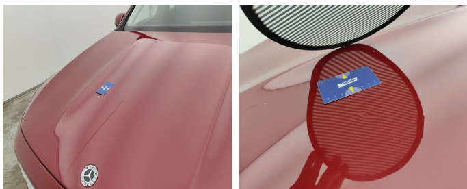
Front Bonnet // Smart Repair Small-dent
