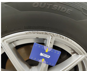
Wheel Alloy Front Right // Repair-scratch
