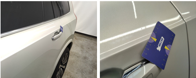
Door Rear Right // Repair & Painting-bad repair
