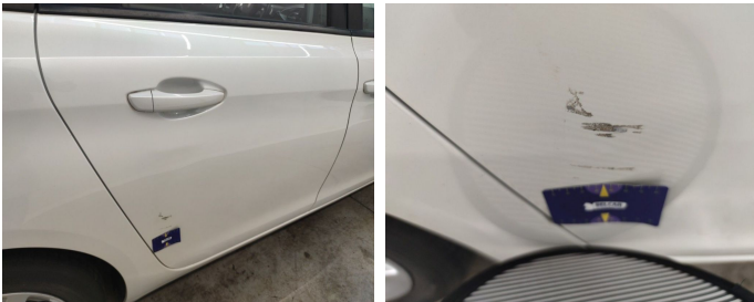
Door Rear Right // Repair & Painting-dent
