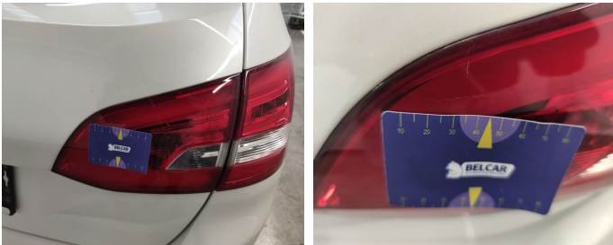
Light / Rear Right On Rear Bonnet / Replace-scratch
