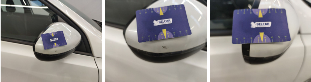
Side View Mirror Right // Painting-scratch
