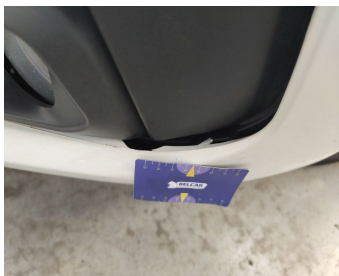
Bumper Front / Trim Left / Replace-cracked
