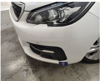
Bumper Front / Trim Left / Replace-cracked
