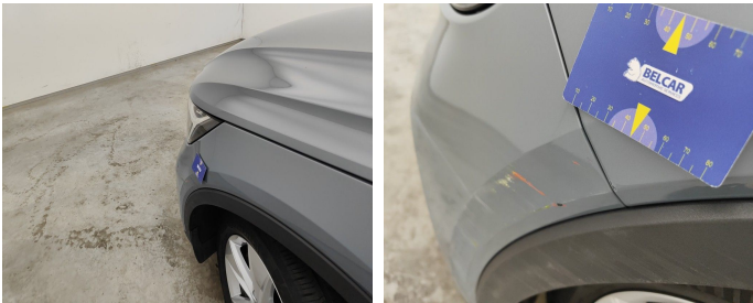
Wing Front Left // Smart Repair Medium-scratch
