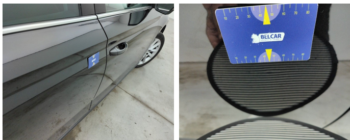
Door Rear Right // Smart Repair Small-dent
