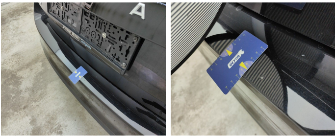
Bumper Rear // Smart Repair Medium-scratch
