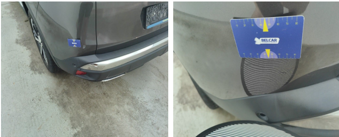
Bumper Rear // Repair & Painting-scratch + dent
