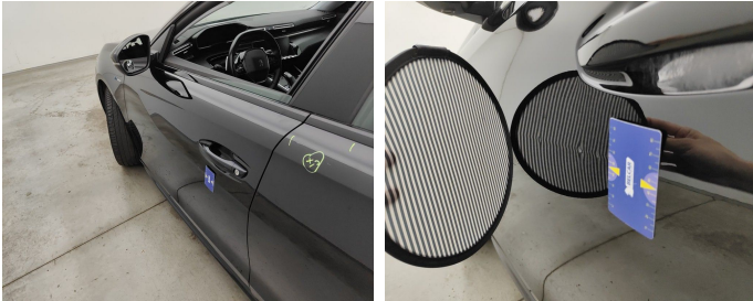
Door Front Left // Repair & Painting-scratch + dent
