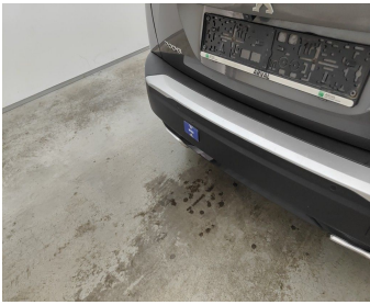
Bumper Rear / Lower Cover Not Painted / Replace-scratch
