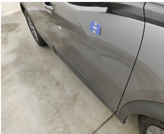
Door Front Right // Repair & Painting-scratch + dent
