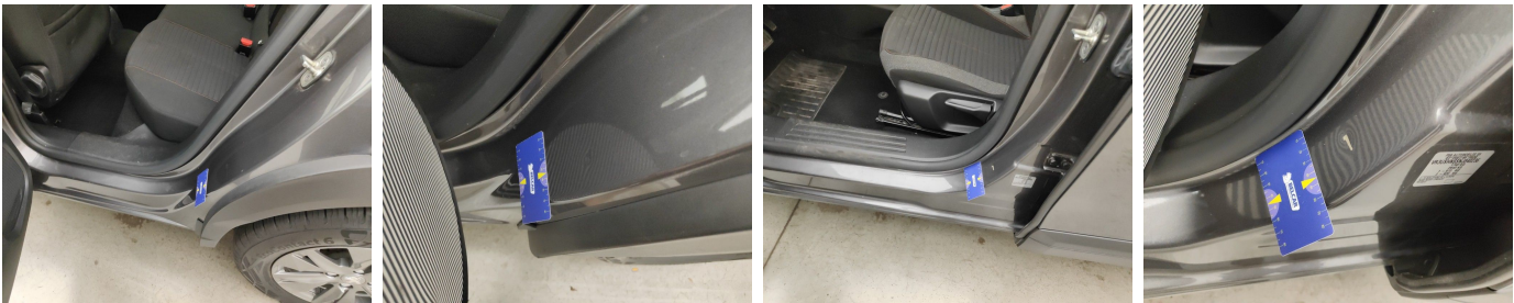
Rocker Panel Left // Smart Repair Medium-scratch + dent
