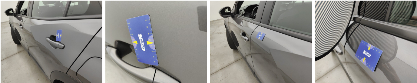
Door Rear Left // Repair & Painting-scratch + dent
