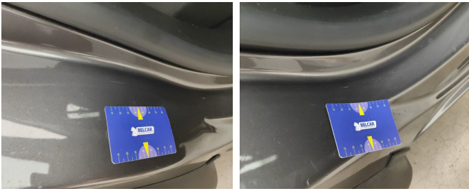
Rocker Panel Right // Smart Repair Medium-scratch + dent
