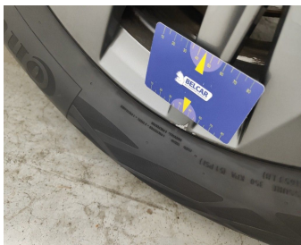
Wheel Alloy Front Right // Repair-scratch
