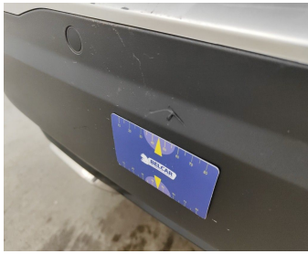
Bumper Rear / Lower Cover Not Painted / Replace-scratch
