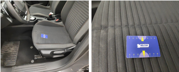
Seat Front Left / Bottom Coating / Replace-Incinerated
