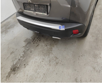
Bumper Rear / Trim Center / Replace-scratch
