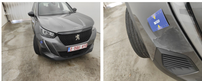
Bumper Front // Painting-Chipped paint
