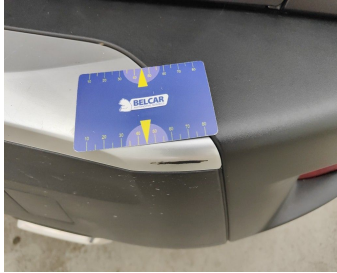
Bumper Rear / Trim Center / Replace-scratch
