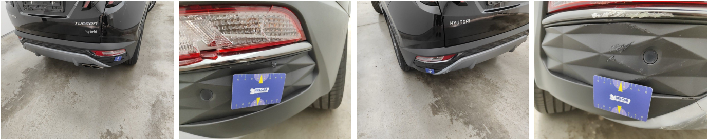
Bumper Rear / Trim Center / Replace-scratch
