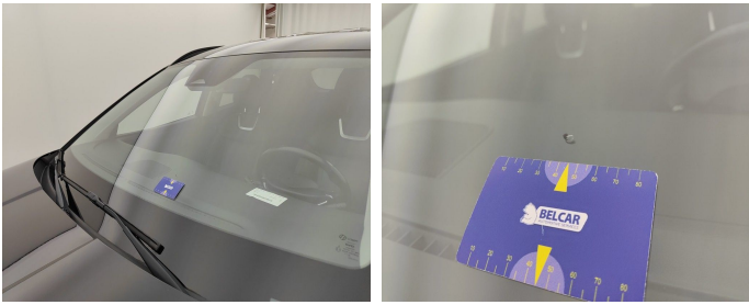
Windshield // Repair-glass damage
