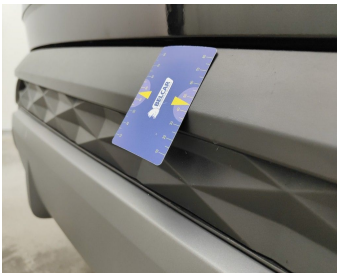
Bumper Rear / Lower Cover Not Painted / Replace-cracked
