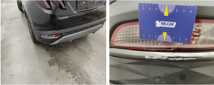
Back Side / Reflector L / Replace-scratch
