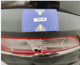
Back Side / Reflector R / Replace-cracked
