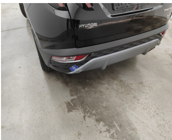
Bumper Rear / Lower Cover Not Painted / Replace-cracked
