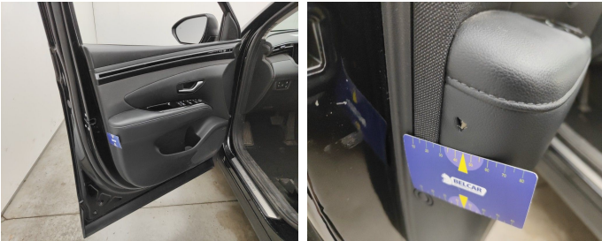
Front Left Door Interior Coating // Replace Completely-hole
