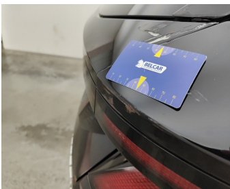
Wing Rear Right // Repair & Painting-scratch + dent
