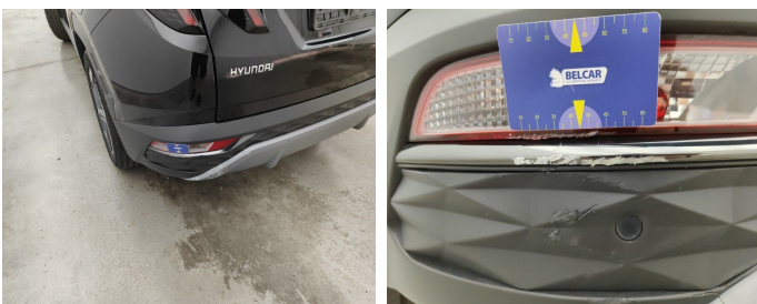
Bumper Front / Lower Cover Not Painted / Replace-scratch
