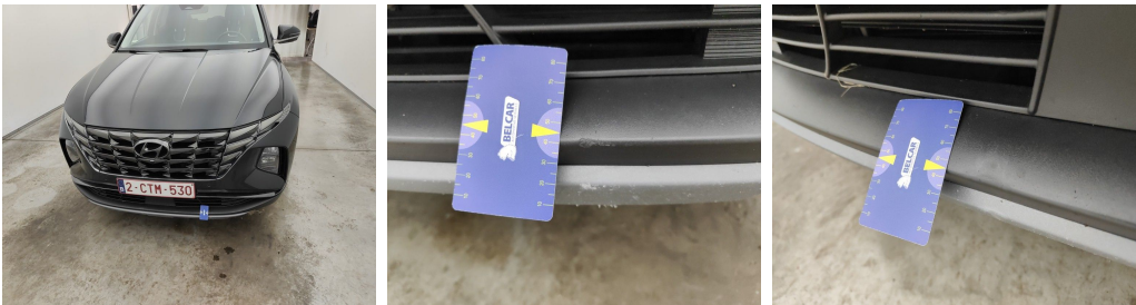
Bumper Front / Lower Cover Not Painted / Replace-scratch
