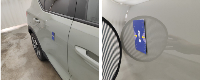
Door Rear Right // Repair & Painting-scratch + dent
