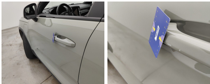
Door Front Left // Smart Repair Medium-scratch
