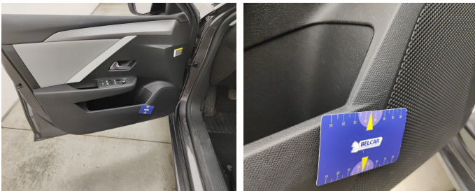
Front Left Door Interior Coating // Replace Completely-scratch
