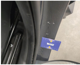
Rocker Panel Left // Smart Repair Medium-scratch + dent
