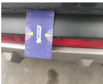
Bumper Rear / Lower Cover Not Painted / Replace-scratch
