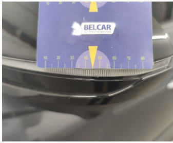
Side View Mirror Left / Direction Indicator / Replace-scratch
