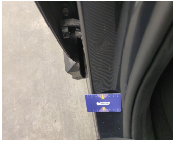
Rocker Panel Right // Smart Repair Medium-scratch + dent
