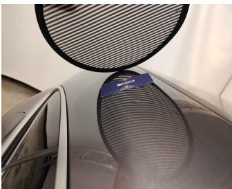
Roof // Smart Repair Medium-dent
