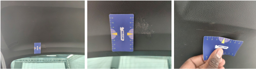
Trunk Lid Interior Coating / Complete Panel / Replace-scratch
