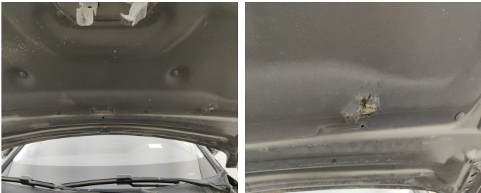
Front Bonnet / Insulation / Replace-hole
