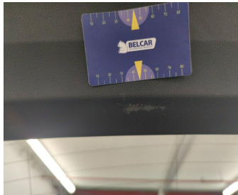
Trunk Lid Interior Coating / Complete Panel / Replace-scratch
