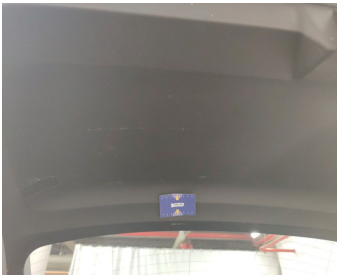
Trunk Lid Interior Coating / Complete Panel / Replace-scratch
