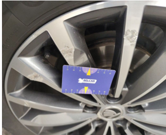
Wheel Two Tone Front Right // Repair-scratch
