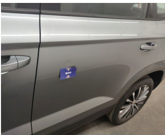
Door Rear Left // Repair & Painting-scratch + dent
