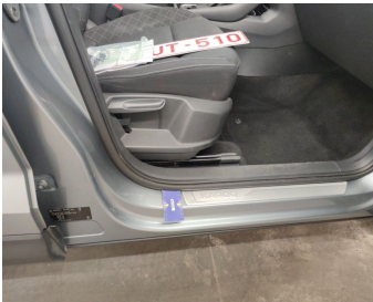
Rocker Panel Right / Cover Not Painted / Replace-dent
