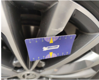
Wheel Two Tone Front Left // Repair-scratch
