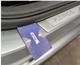
Rocker Panel Right / Cover Not Painted / Replace-dent
