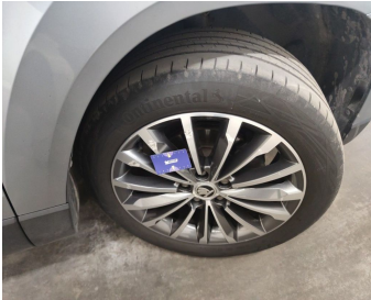
Wheel Two Tone Front Right // Repair-scratch
