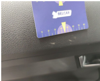
Rear Left Door Interior Coating // Replace Completely-scratch
