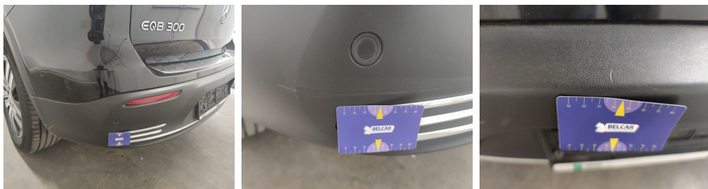
Bumper Rear / Lower Cover Not Painted / Replace-scratch
