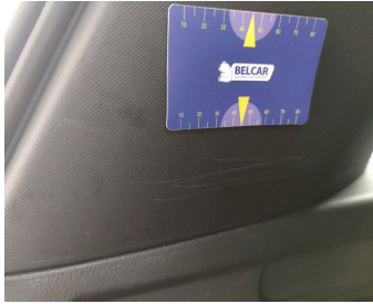
Trunk Compartment / Side Cover Left / Replace-scratch
