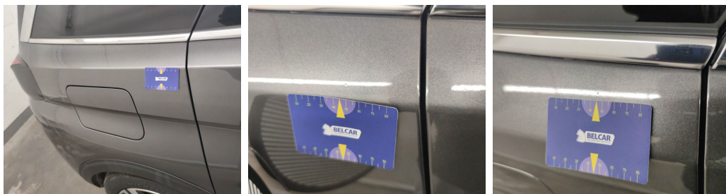
Wing Rear Right // Painting-bad repair
