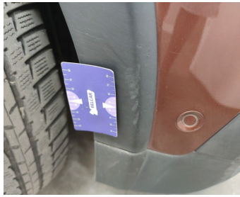
Bumper Front / Trim Right / Replace-scratch
