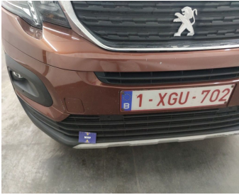
Bumper Front / Spoiler / Replace-scratch
