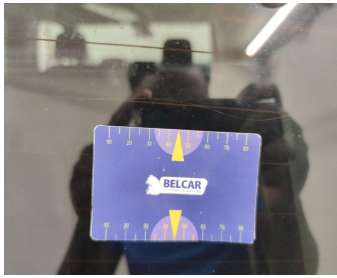
Rear Bonnet / Rear Window / Replace-scratch
