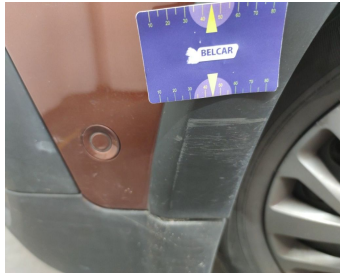
Bumper Front / Trim Left / Replace-scratch
