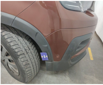
Bumper Front / Trim Right / Replace-scratch
