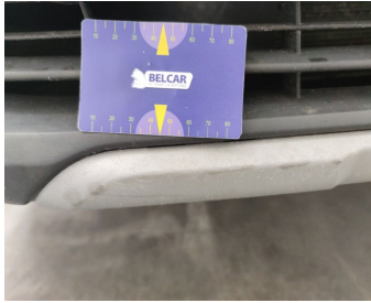
Bumper Front / Spoiler / Replace-scratch
