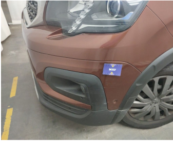
Bumper Front / Trim Right / Replace-scratch
