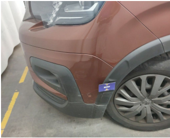
Bumper Front / Trim Left / Replace-scratch
