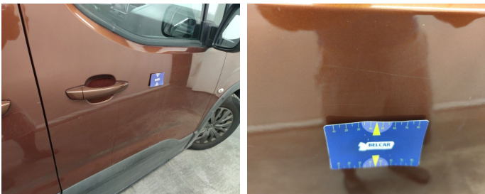
Door Front Right // Polish-scratch
