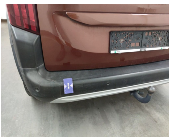
Bumper Rear // Replace without painting-scratch
