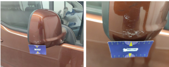
Side View Mirror Right // Painting-scratch
