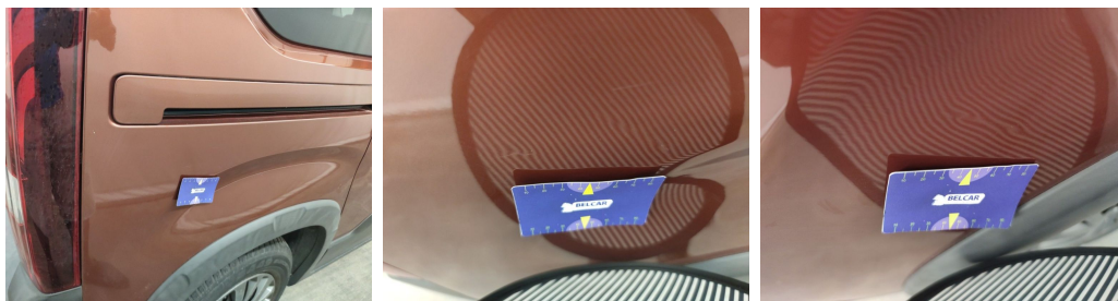
Wing Rear Right // Repair & Painting-scratch + dent
