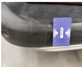
Bumper Rear // Replace without painting-scratch
