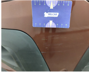
Bumper Front / Trim Right / Replace-scratch
