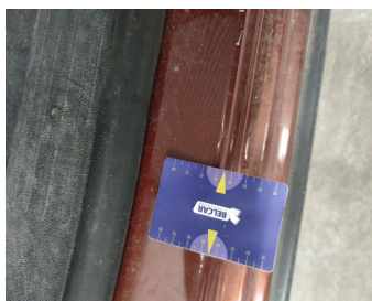
Bumper Rear // Replace without painting-scratch
