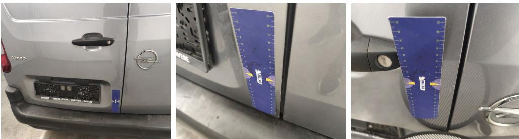
Rear Loading Door Right // Repair & Painting-scratch + dent
