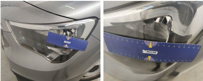
Headlight / Front left / Replace-scratch
