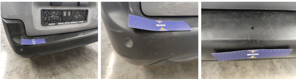
Bumper Rear / Lower Cover Not Painted / Replace-scratch
