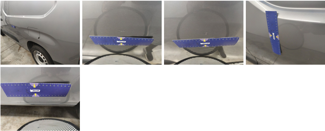
Wing Rear Left // Repair & Painting-scratch + dent
