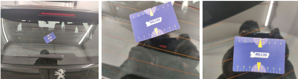
Rear Bonnet / Rear Window / Replace-scratch
