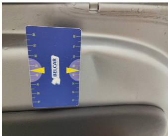
Rear Bonnet // Repair & Painting-scratch + dent
