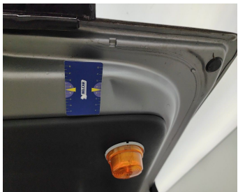
Rear Bonnet // Repair & Painting-scratch + dent
