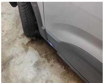
Rocker Panel Left // Repair & Painting-scratch + dent
