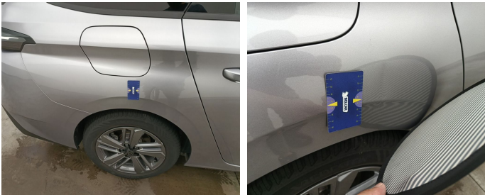
Wing Rear Right // Repair & Painting-scratch + dent
