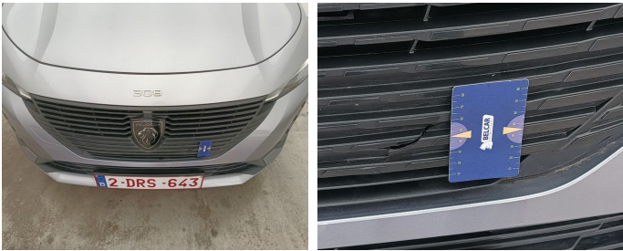
Front / Calendar / Replace-cracked
