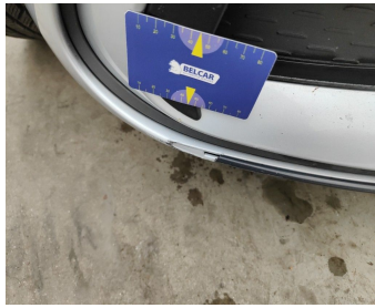
Bumper Front / Trim Right / Replace-cracked
