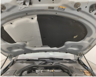
Front Bonnet / Insulation / Replace-tear
