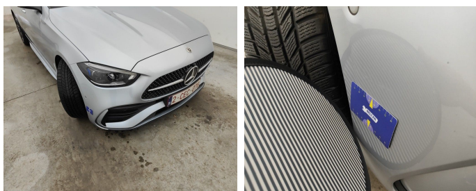
Bumper Front // Smart Repair Large-scratch + dent
