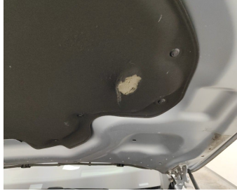
Front Bonnet / Insulation / Replace-tear
